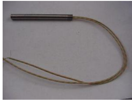
Figure 4.2 Cylindrical Cartridge Heat Source
